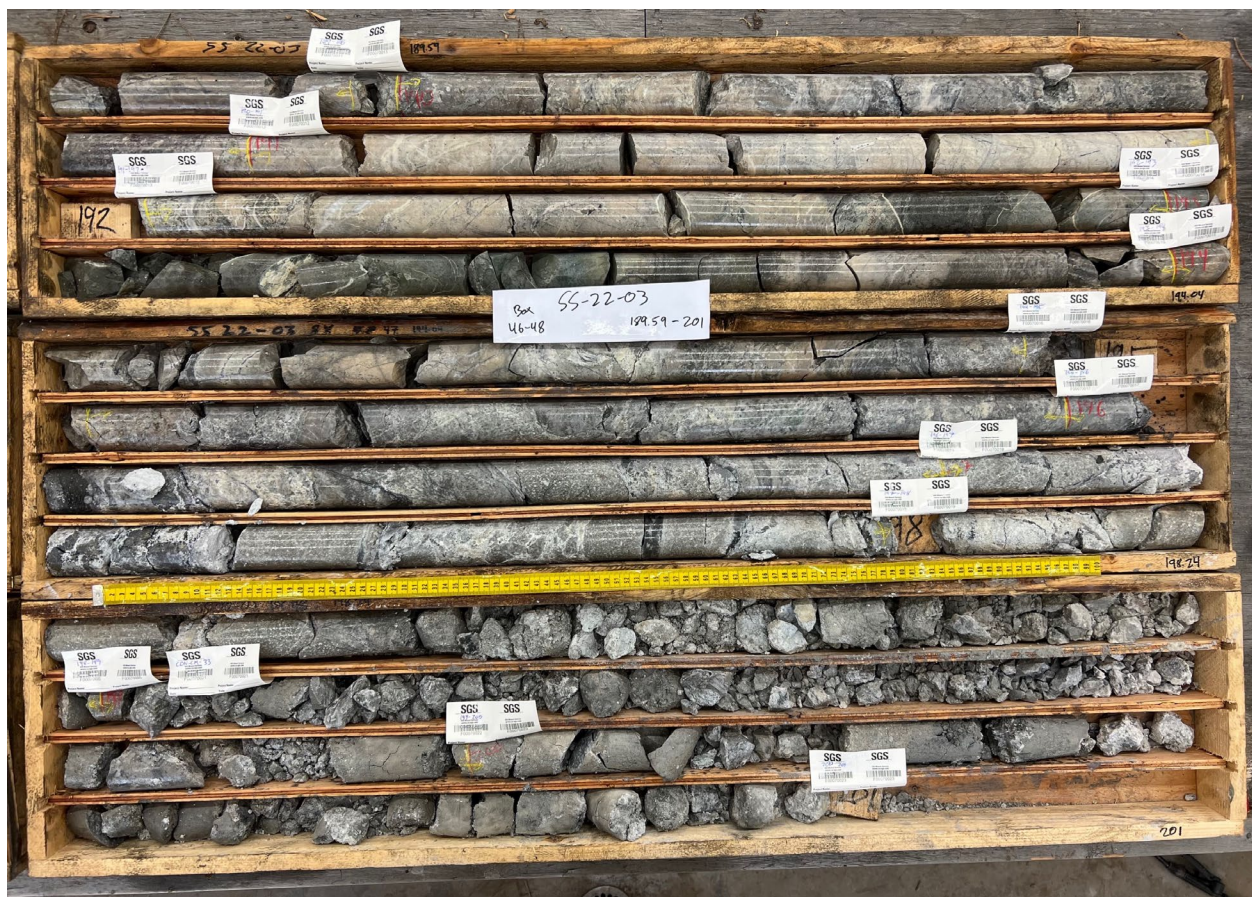
Figure 6-4 Drill Core from SS-22-03 from 189.59 – 201.00 m consisting of well mineralized and strongly altered fine grained volcanics. Mineralization consists of up to 20% pyrite, sphalerite and galena as semi massive lenses, veins and pervasively disseminated fine to medium grained sulphide grains.
